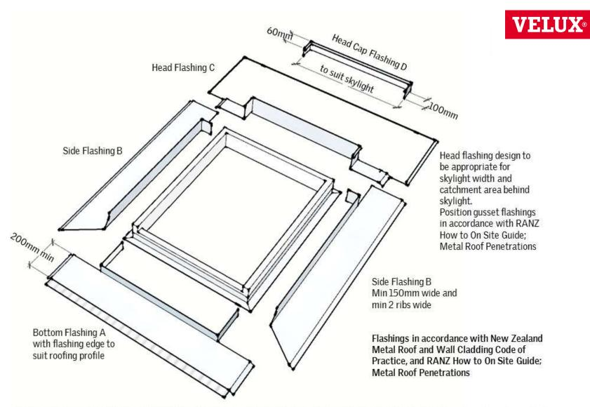
UNDER SOAKER CUSTOM FLASHING DETAIL for ROOF PITCHES OVER 15 DEGREES (Guide only - Check on site)
