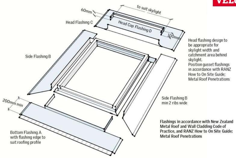
CUSTOM OVER FLASHING DETAIL for ROOF PITCHES OVER 15 DEGREES (Guide only - Check on site)
